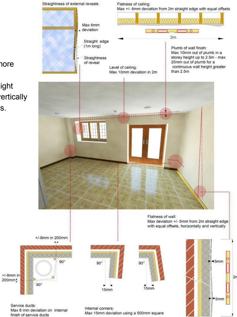
Figure 6: Maximum deviation in walls and ceilings
