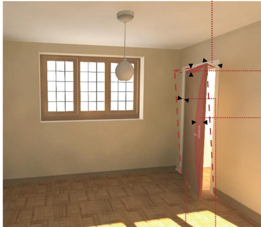
The gap between the underside of an internal door and unfinished floor (concrete, screed, etc) should be min 5mm and max 22mm
