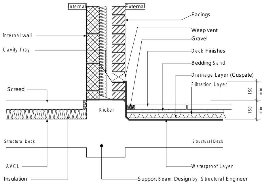
**Podium deck – wall waterproofing detail (Bedded slabs)**
