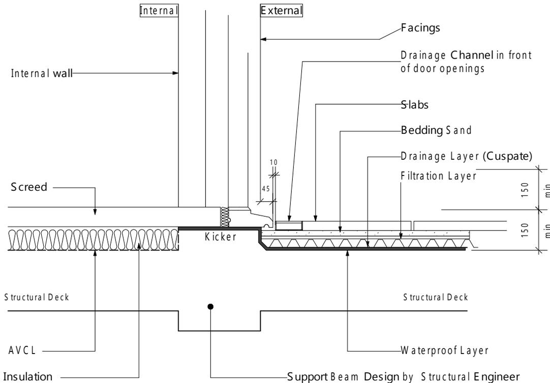
**Podium deck – Threshold waterproofing detail (bedded paviers)**
