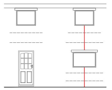
Movement joints should not pass through openings due to the difficulty in continuing the joint between the frame and masonry and around the end of lintels.
