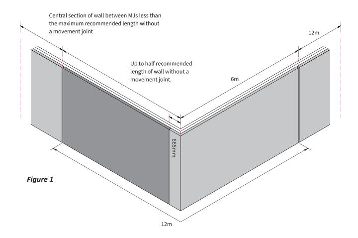
Short returns in clay masonry (less than 675mm) should have movement joints as per figure 2 below. Movement joints can be specified with the use of a 'compressible joint' or a 'slide by joint'.
