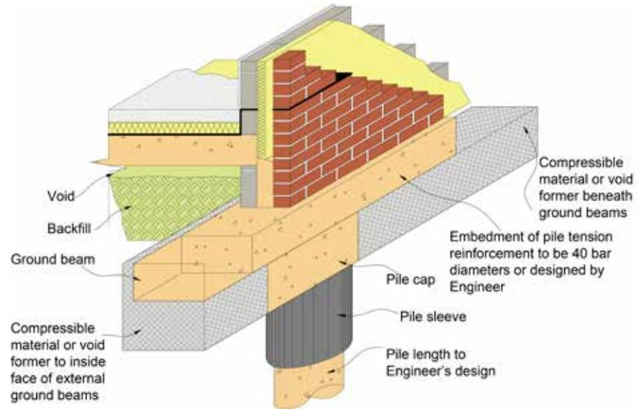
Figure 10: Heave protection: Section of pile and beam foundation
