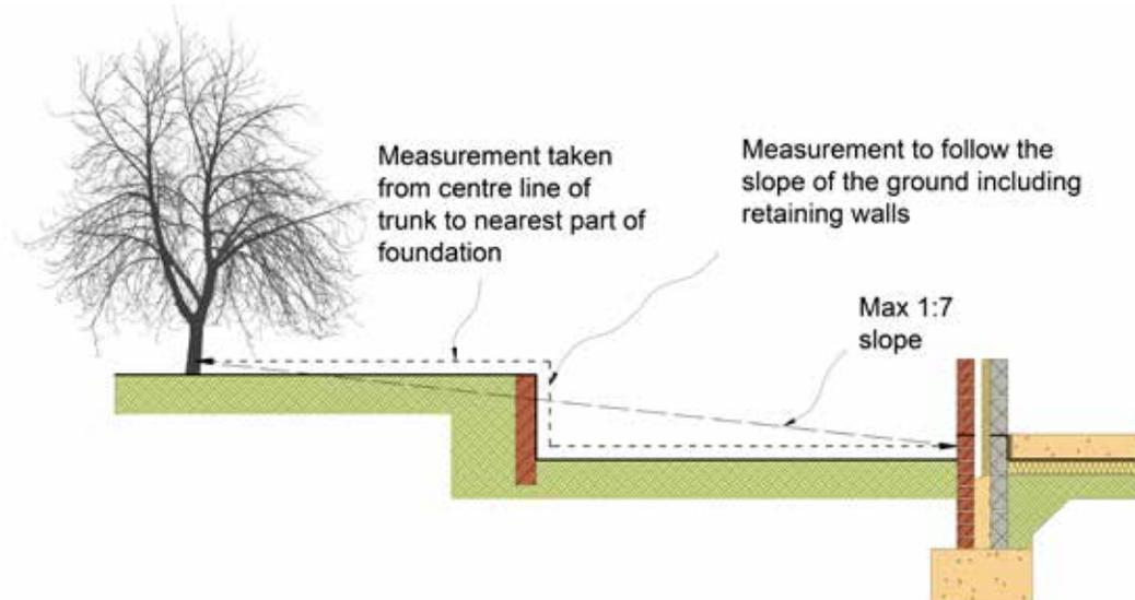
Figure 11: Measuring foundation distance on sloping sites
