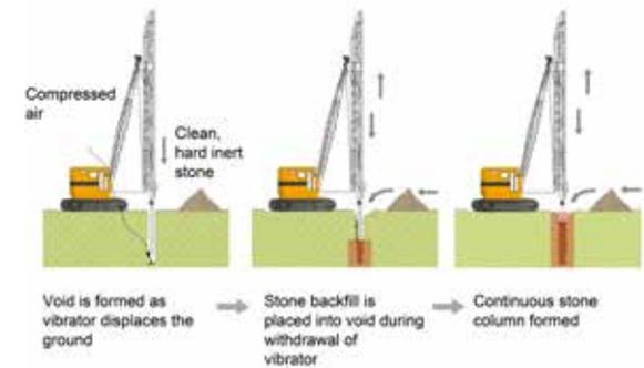
Figure 1: Vibratory techniques: dry bottom feed method
