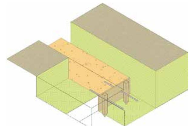
Figure 16: Using reinforcement bars across a joint
