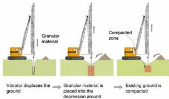
Figure 2: Vibratory techniques: dry top feed method
