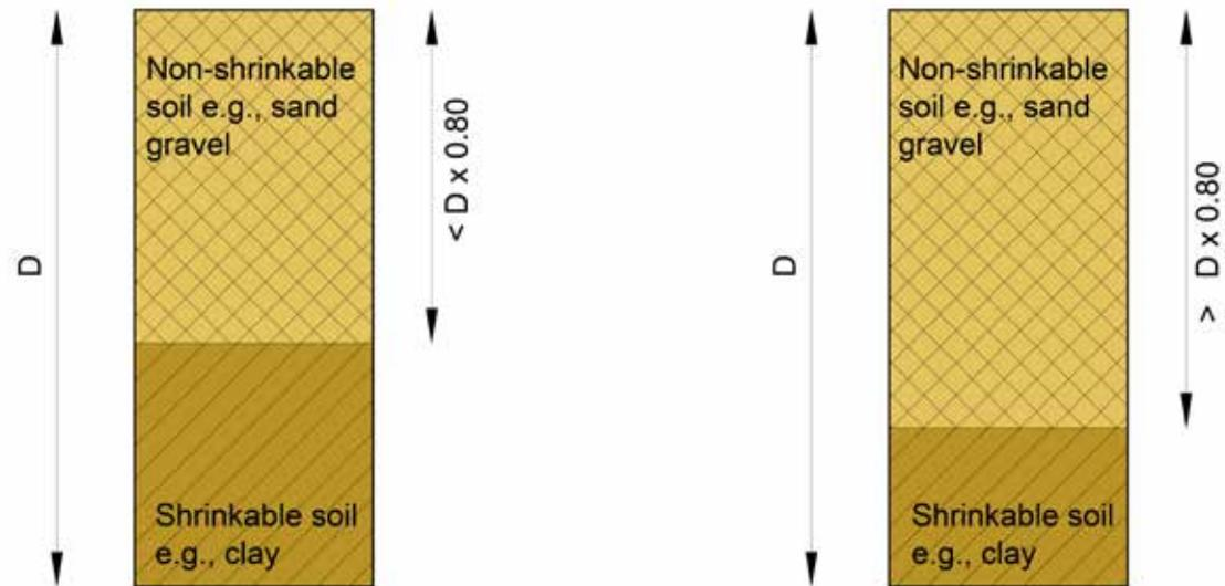
Figure 12 and 13: Foundation depth required to be taken down using foundation calculator and plasticity index of underlying clay
