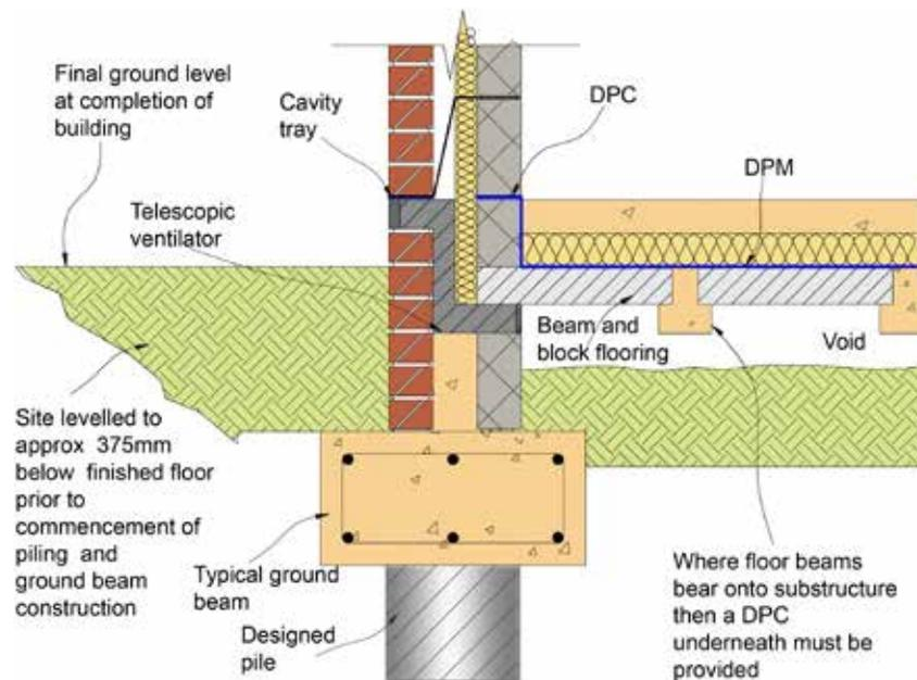
**Figure 19: Pile and beam detail**
