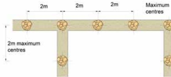
Figure 4: The intersection of adjacent reinforced concrete strips
