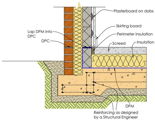
Figure 20: Typical raft foundation design
