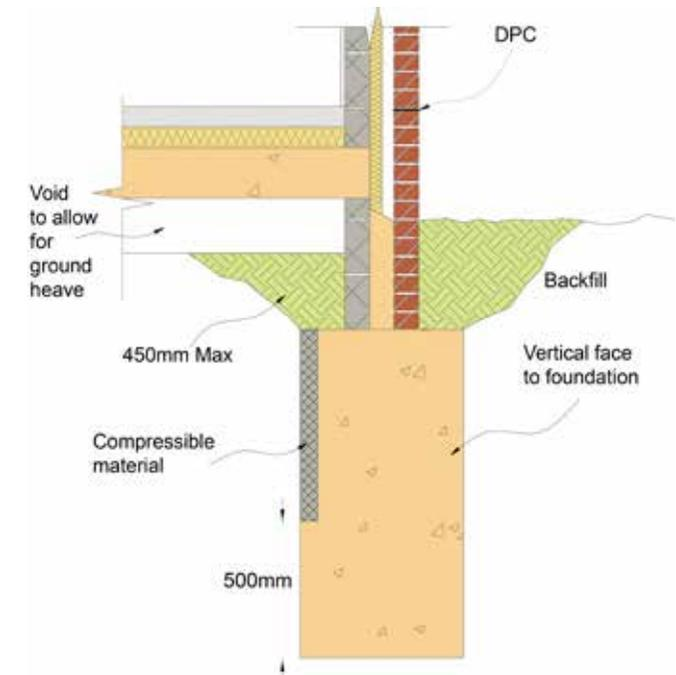
**Figure 8: Heave protection: Section through a typical mass filled foundation**
