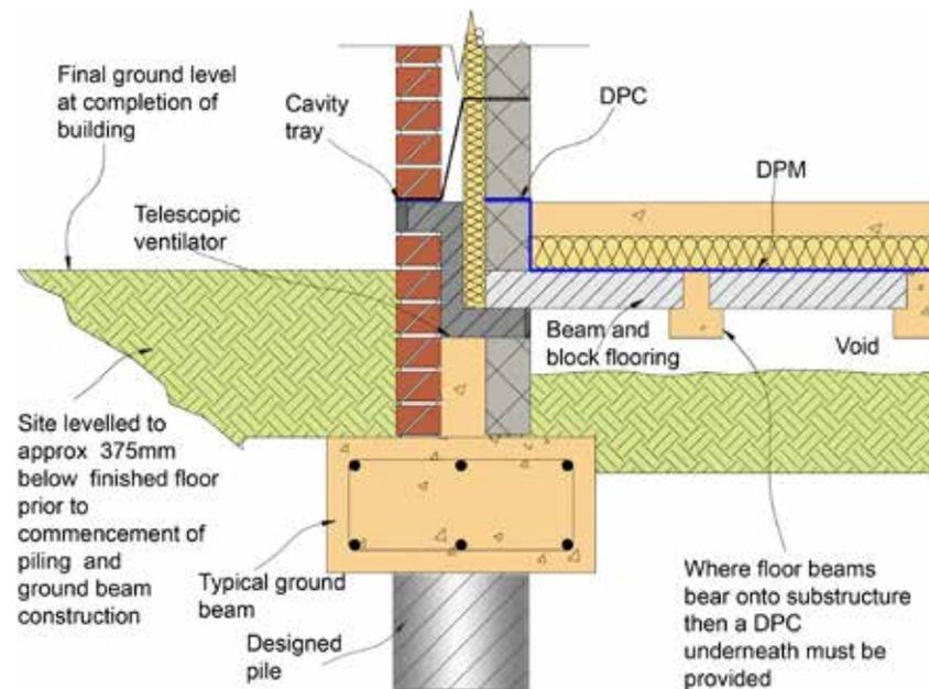
Figure 19: Pile and beam detail
