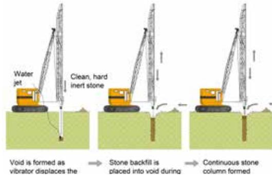
Figure 3: Vibratory techniques: wet bottom feed method
