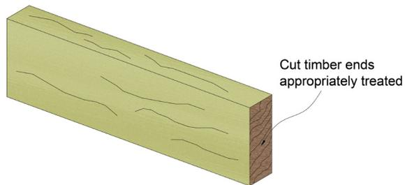
Figure 2: Pre-treated timber exposing untreated end grain
