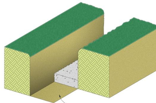
Concrete should not be poured if ground is frozen and if temperature is less than 2 °C
