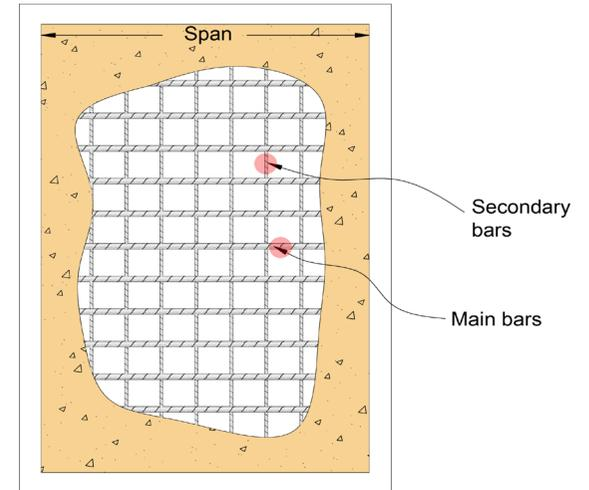
Figure 8: Position of bars on reinforced concrete slab
