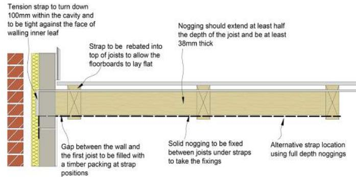
Figure 6: Lateral restraint to floors
