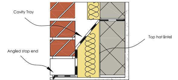
Figure 19: Stop-end in relation to cavity tray and lintel
