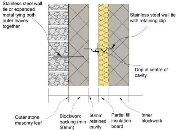
Figure 24: Masonry cavity wall with stone outer leaf
