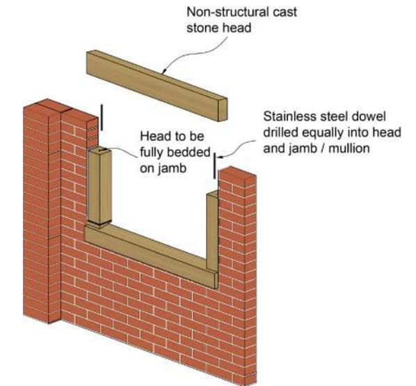
Figure 26: Joining stone jambs to sills and head
