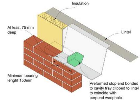
Figure 18: Stop-end to cavity tray
