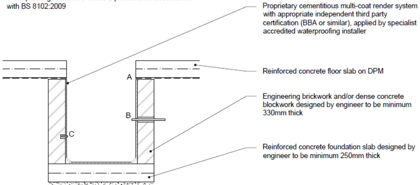
The following waterproofing details must be installed in accordance with a specialist design using proprietary products that are compatible with the multi-coat render system:
