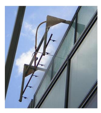
Spray bar testing is suitable for open-jointed systems (e.g. rainscreen cladding and unsealed patent glazing) and opening joints, as water is not forced into the joint.
