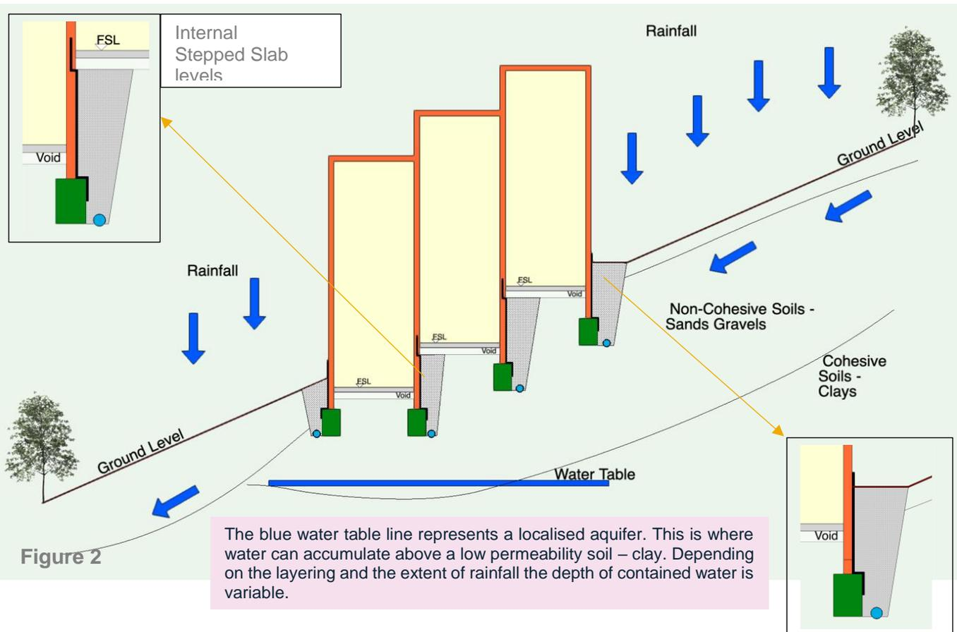
Ground floor slabs and environments must be protected from the ingress of groundwater and damp where they are located below the external ground level. Two methods are available which can effectively protect ground slab and environment when located below the external ground level.
