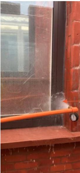
Example of hose testing completed to panelised system in factory, prior to required onsite testing.
