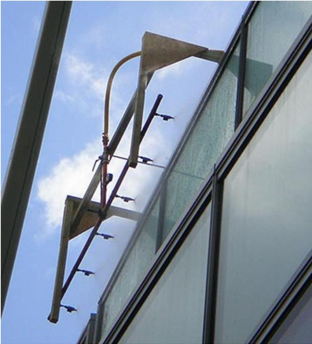
**\*Spray bar testing is suitable for opening joints in curtain walling and sealed interfaces prior to rainscreen cladding being installed.**
