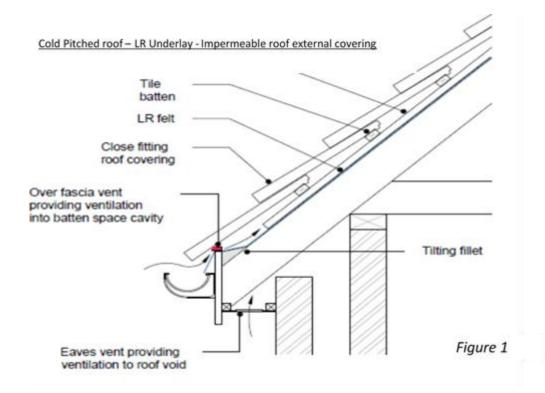
If the batten space is not ventilated, there needs to be an increased level of ventilation to the roof space and that should be in accordance with BS5250. The underlay manufacturer's 3rd party accreditation also needs to be followed. It is very difficult to determine a HR or LR underlay by sight alone and the manufacturer's third party accreditation should be referred to.
