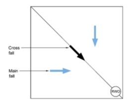
**Interrupted falls** – the position directly behind roof lights often gives rise to the opportunity for slowed drainage or drainage 'dead spots' where water ponds due to interruption of the roof fall. Drainage crickets are double triangle structures, constructed in the deck or sometimes provided by insulation to divert water around obstructions. Where these are not supplied, ponding will often occur.
