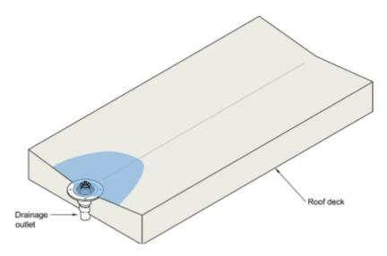
**Sumps and gutters** – during a storm event these will fill extremely fast until the design head is reached. Once the equilibrium state is reached, with the water discharging down the outlets to match the rate of water arriving, sumps and gutters should then be free of standing water. The depth of a sump or gutter should be 25mm above the design head of water. Ponding water should not overtop the defined edge of the sump or gutter and spill out onto the roof slope.
