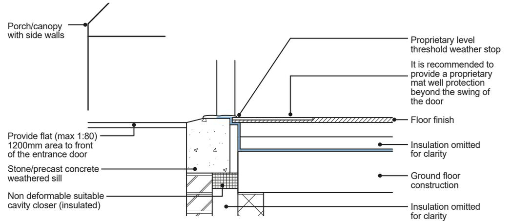
**Typical level threshold without canopy protection**
