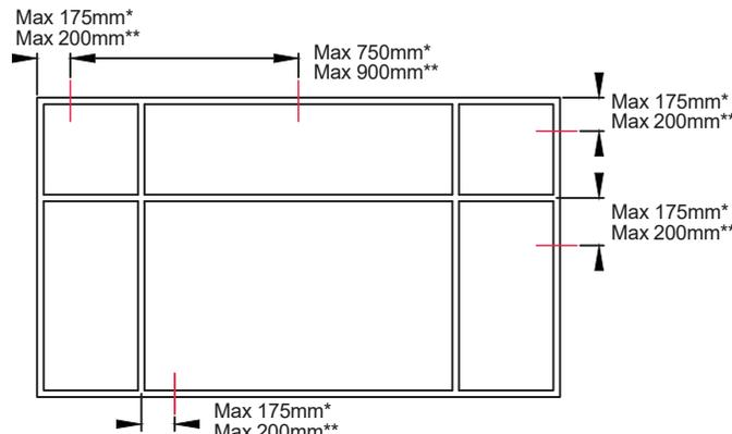
\* Dimension for hot rolled sections
