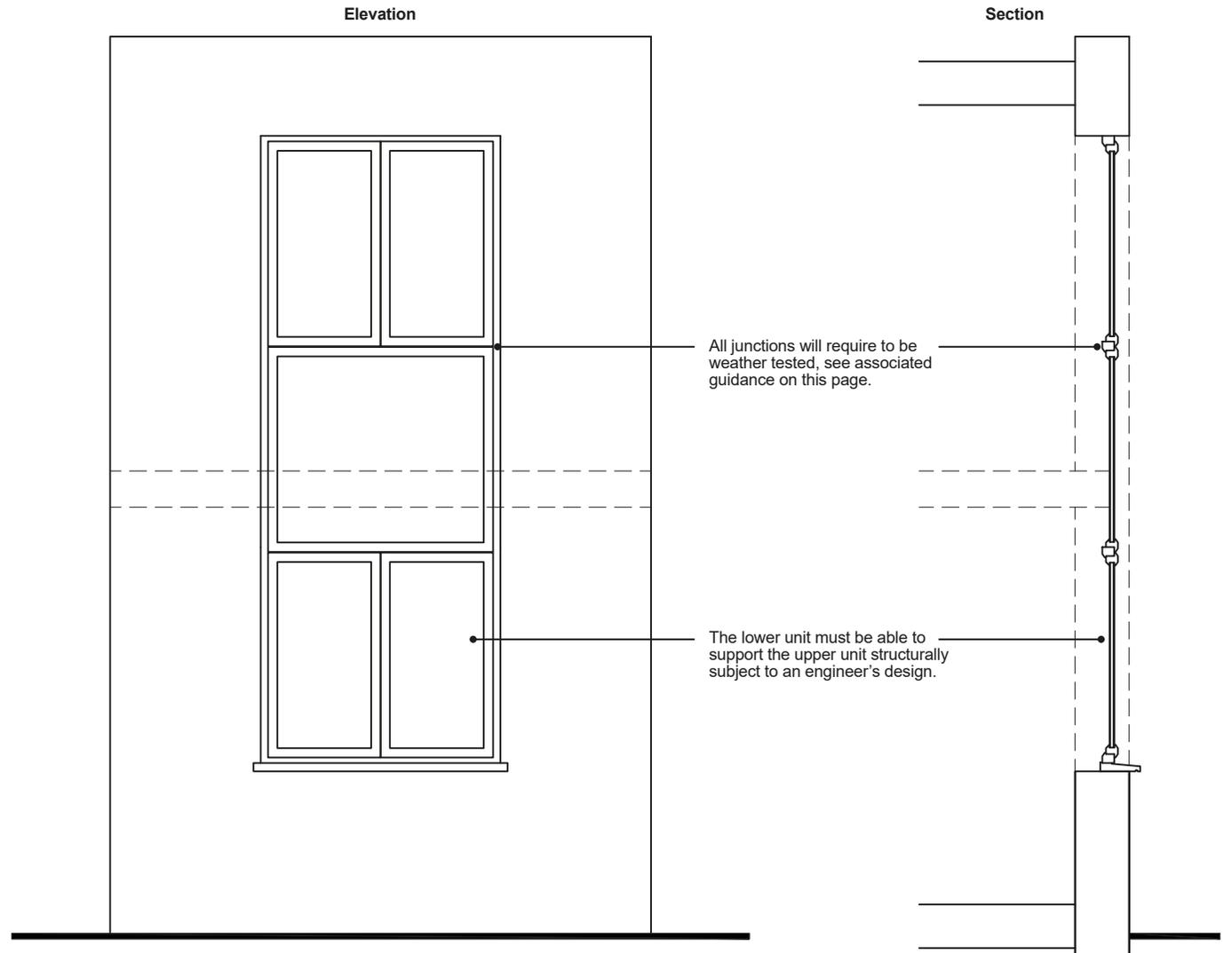
Fixing should allow for differential movement if in a timber framed building as well as suitability to join one frame to the other. Fixings must also meet the requirements of BS8213: 4 for spacing requirements with particular emphasis on the side and tops.
