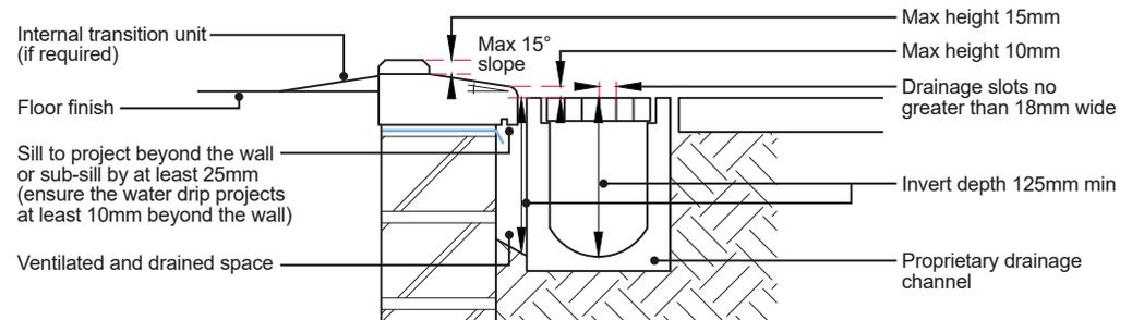
These illustrations show accepted practice for forming a weather resistant threshold detail and may not indicate the full extent of insulation requirements to meet relevant Building Regulations.
