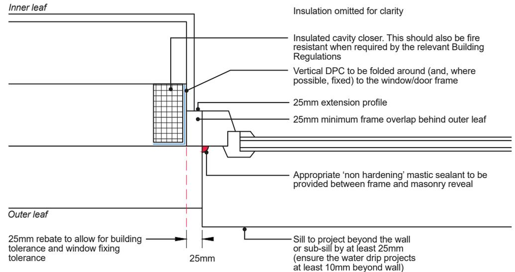
When installing window/door frames in a checked rebate, allow for the frame to be deeper:
