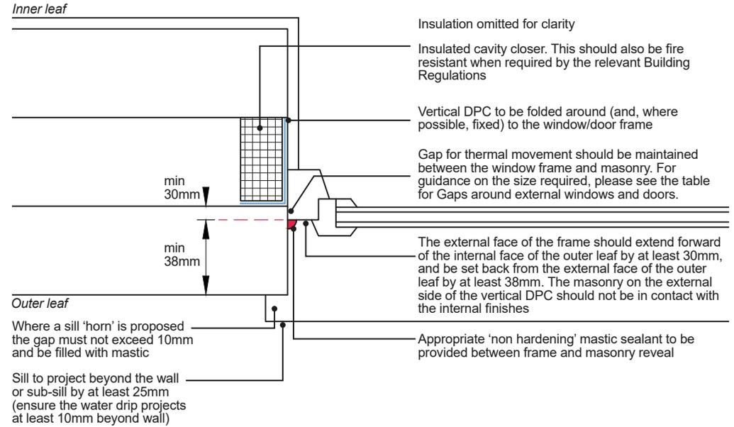
**Checked rebate window frame detail for areas of very severe exposure**
